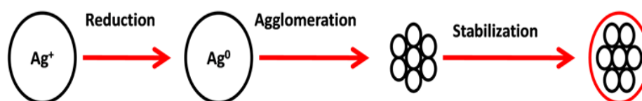
Fig. 1. A schematic diagram showing the silver ion reduction, agglomeration and stabilization to form a particle of nano size
