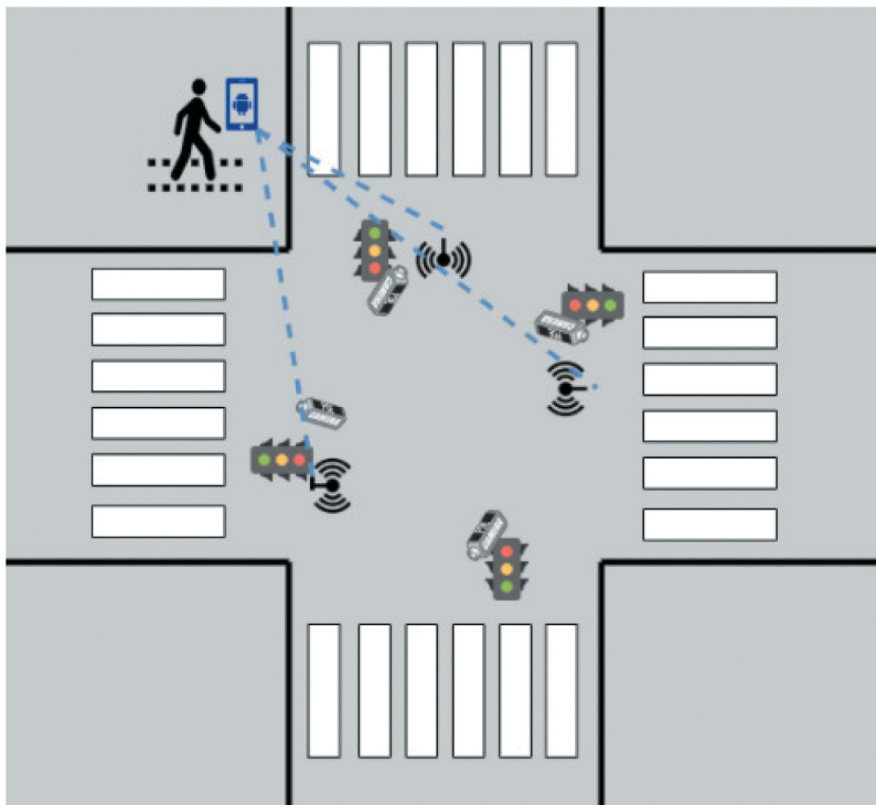
Figure 1. Proposal of camera and smart traffic lights installation in an intersection.
