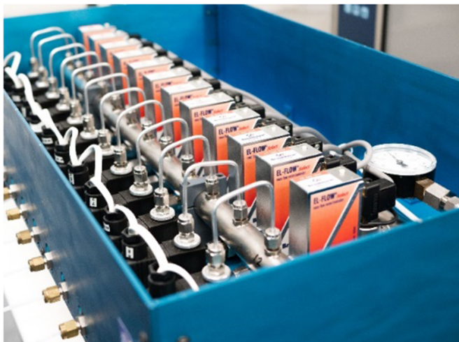
Figure 3. Sampling manifold with valves and MFCs.
