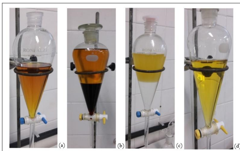
Fig. 3. Steps in the production of biodiesel from filtered frying oil (a) Filtered frying oil (b) Separation of phases – impure glycerine in the bottom and impure biodiesel on the top (c) Purification step – washing with water (d) Purified biodiesel
