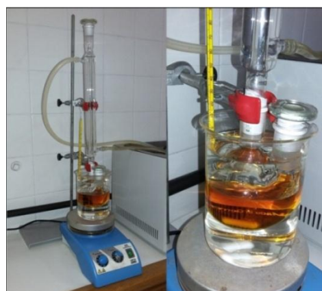
Fig. 2. Assembling of the reaction system for the production of biodiesel
