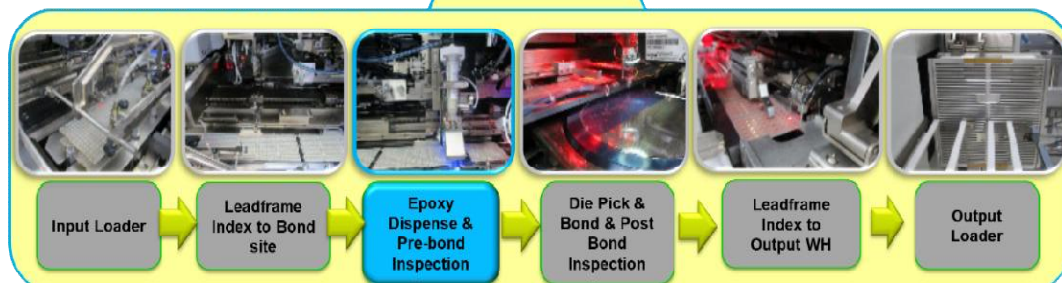
Fig. 3. Die attach process mapping
