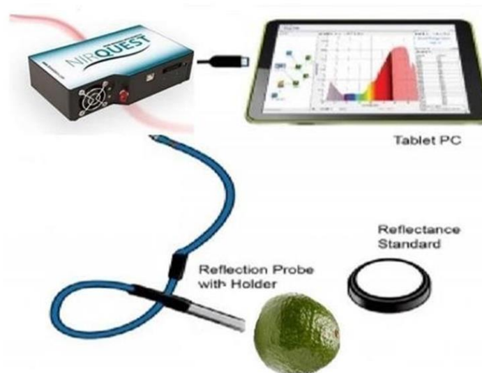
Fig. 1. Set-up for diffuse reflectance of Hass avocado samples
