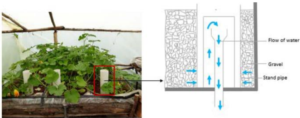
Fig. 2. Schematic layout of a hydroponic unit with a bell siphon
