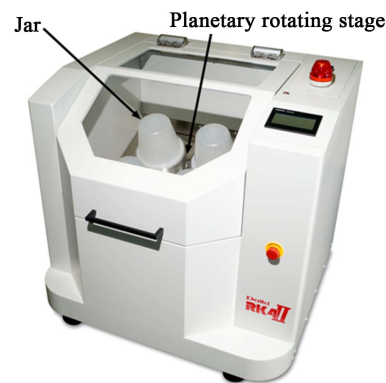
Figure 1. The developed rod mill (DIK-2610, Daiki Co.), which is free from soil dust and has a function of collection of soil particles with a median size of less than 2 mm in diameter.
