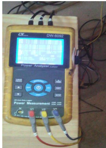
Fig. 1. Lutron 3 Phase digital Power Analyser/meter
