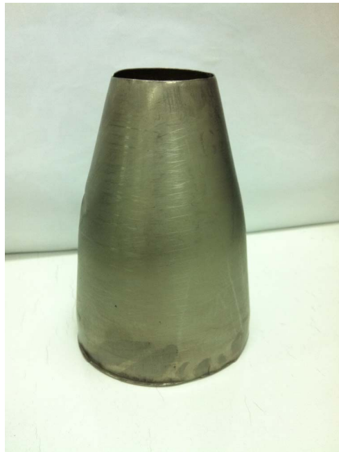
Figure 3. Deformed titanium blank in bulge forming process.
