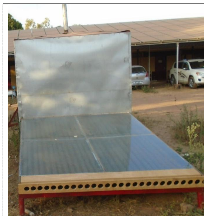
Fig. 3. Solar collector connected to the drying chamber
