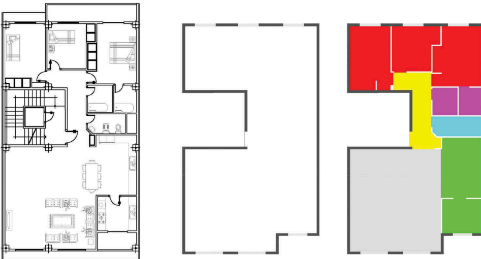
Figure 5. Labeling the Floor plans for cGAN training (Left: Original plan, Middle: Input image, Right: labeled output image).
