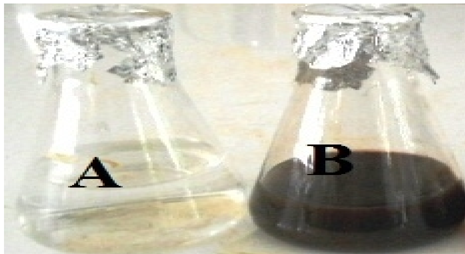
Fig. 2. A Photograph showing aqueous solution of 1mM \text{AgNO}_3 with A. Conyzoides L. plant extracts before adding the different plant extracts (a) and after addition of Water (b)
