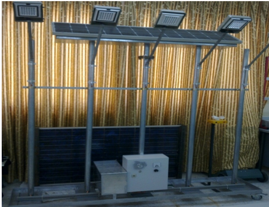
Fig. 10. Practical prototype PV lighting system
