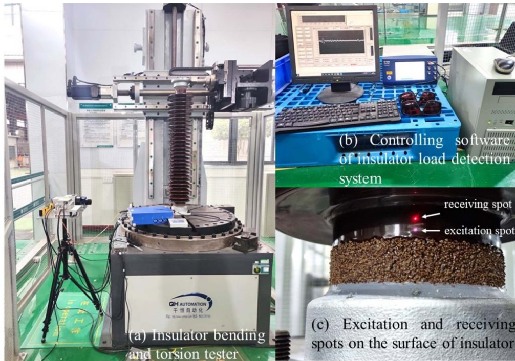
Figure 6. Photographs of the pillar porcelain insulator load detection system based on laser ultrasound.
