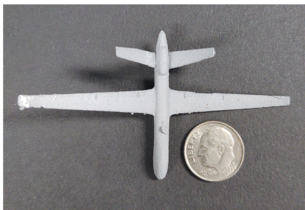
Figure 2. 3D-printed and painted titanium UAV model.
