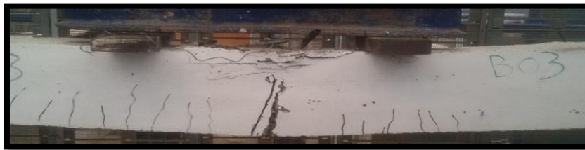
Fig. 8. Crack Pattern of Group A, a) Beam B02; b) Beam B03.
