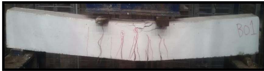
Fig. 7. Crack Pattern of Control Beam B01
