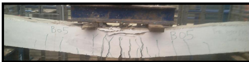
Fig. 9. Crack Pattern of Group B, a) Beam B04; b) Beam B05.
